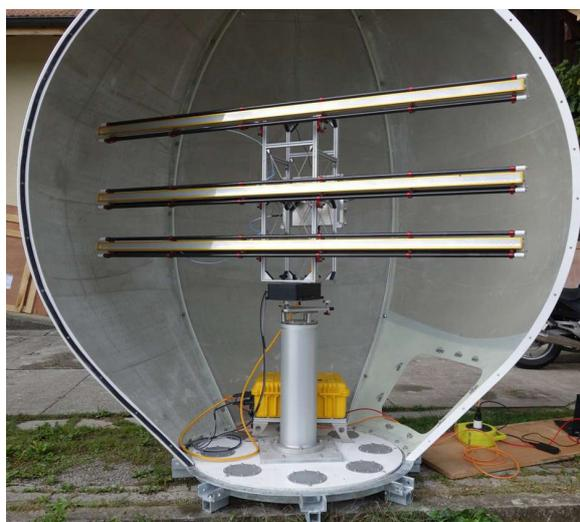
Figure 4: GPRI Radome with steel base.
