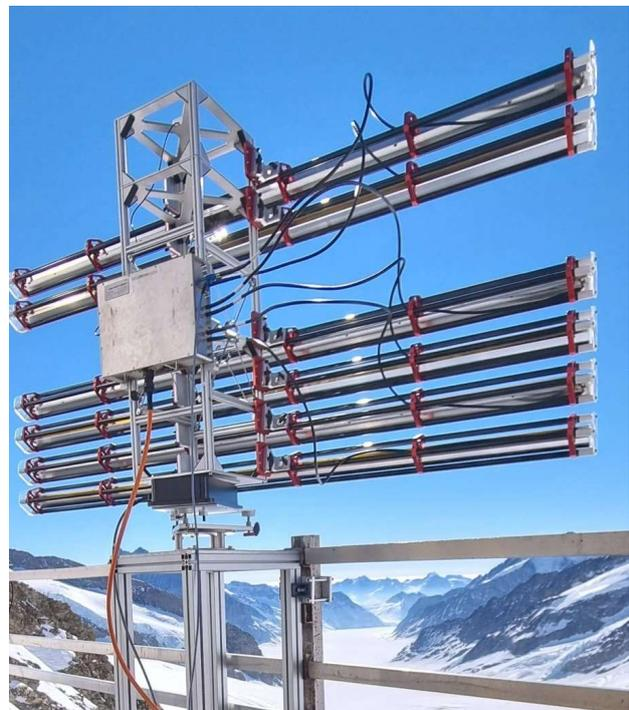
Figure 3: The polarimetric GPRI.
