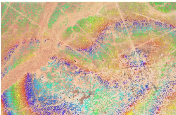
Figure 2 PALSAR SBAS-style displacement time series demo results over an oil field in Oman.
