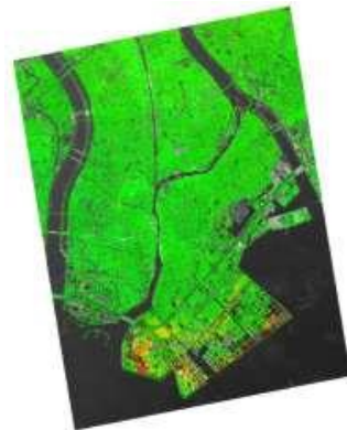
PALSAR-1 PSI example over Chiba, Japan. The average deformation rate is shown using a color scale between -2.5cm/year (red) and +2.5cm/year (blue).
