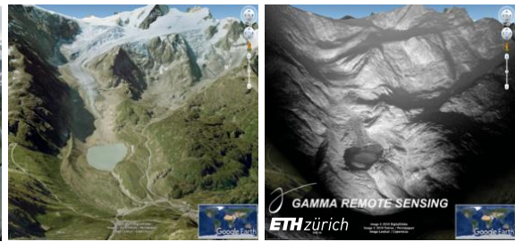
Google Earth view (left) of the Stein Glacier test site (CH). Geocoded intensity image (right) overlaid to Google Earth view as obtained from a car-borne L-band SAR acquisition.
