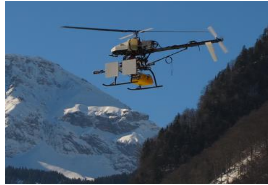
GAMMA L-band SAR on Aeroscout's VTOL UAV Scout B1-100, equipped with a Honeywell HGuide n580 INS/GNSS navigation system, at the test site Wolfenschiessen, Switzerland.
