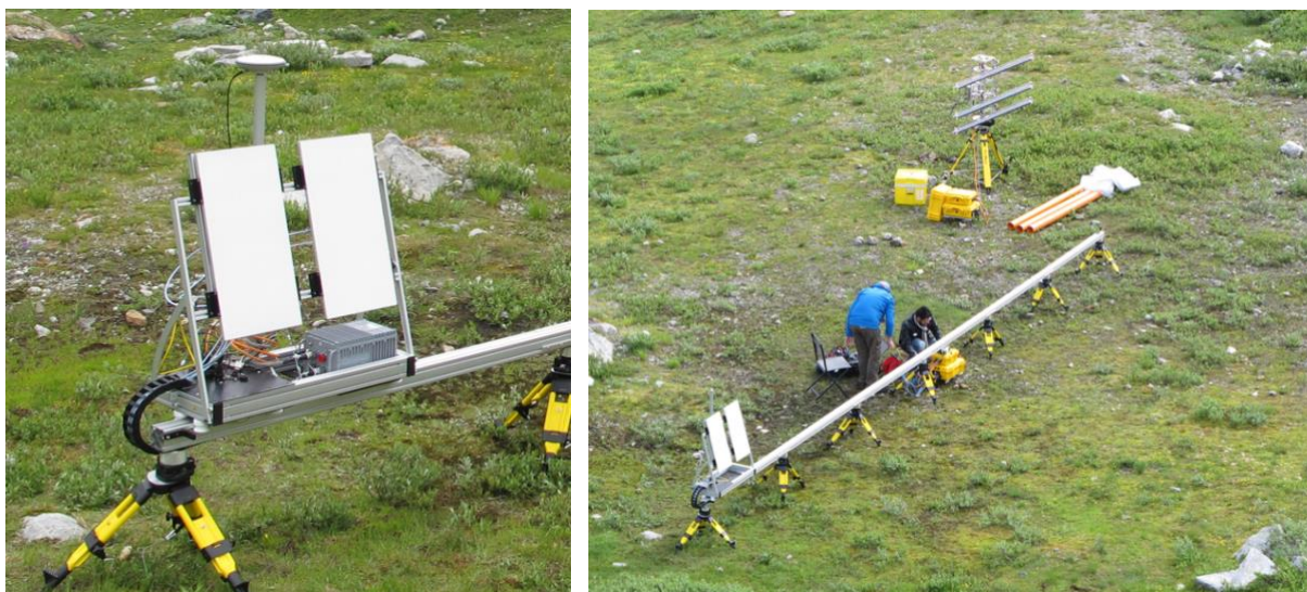
GAMMA L-band SAR mounted on a 12m-long rail for automated repeat-pass InSAR measurements. The rail consists of 6 aluminum profiles of 2m length, each. The system is thus transportable (e.g. in a station wagon, or by helicopter) and it can be mounted by 2 persons in the field. Adjacent to the rail-based GAMMA L-band SAR the Ku-band Gamma Portable Radar Interferometer (GPRI-II) is positioned for comparison.
