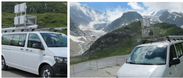
Car-borne setup of the L-band SAR system with one transmit and three receive antennas. Repeated SAR data acquisitions of the Stein Glacier were made while driving on a slightly curved section of mountain road.
