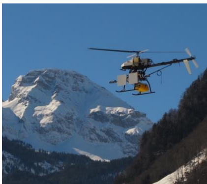
The GAMMA L-band SAR mounted on Aeroscout's UAV Scout B1-100 during an interferometric repeat-pass SAR data acquisition in central Switzerland. The UAV is equipped with a Honeywell HGUIDE n580 INS/GNSS system. GNSS data is processed in post-processing kinematic mode with an ad-hoc local GNSS reference station in the field. SAR antenna/channel configuration: one transmit/ one receive antenna.
