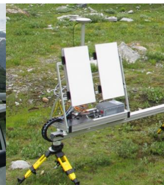
Rail-based terrestrial measurement setup with the GAMMA L-band SAR to autonomously acquire short-interval time series of repeat-pass interferometric SAR data of a glacier.
