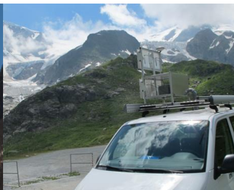
GAMMA L-band SAR mounted on a car during a demonstration campaign in cooperation with ETH Zurich. A ring-laser-gyro INS/GNSS system (iNAV-RQH) by iMAR Navigation GmbH was used for high-precision positioning and attitude determination. GNSS data is processed in post-processing kinematic mode with an ad-hoc local GNSS reference station in the field. SAR antenna/channel configuration: on transmit/ three receive antennas.
