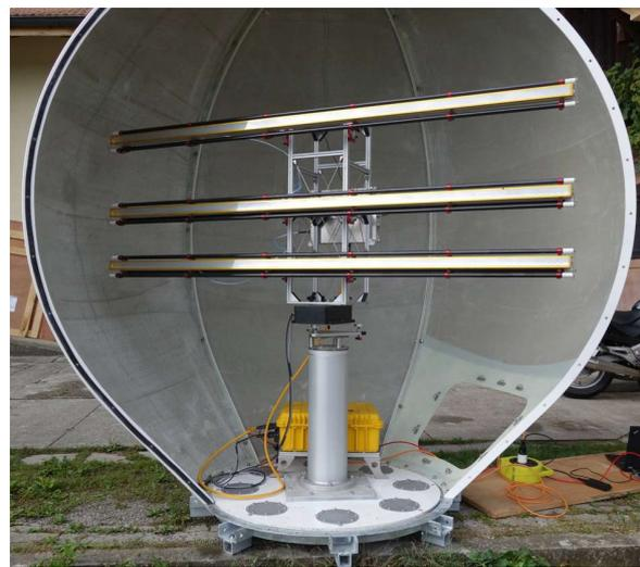
Figure 4: GPRI Radome with steel base.
