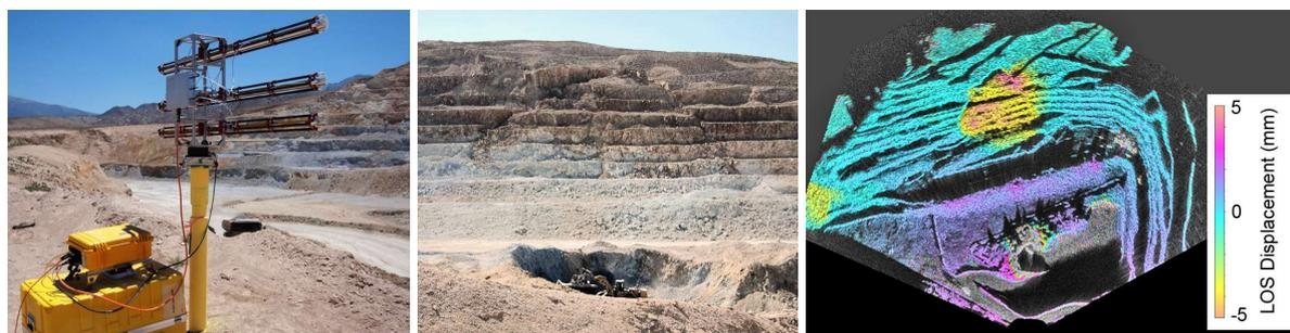
Figure 8: Monitoring of a **slope instability** in the Round Mountain Gold Mine, Nevada, USA, over vegetation-free terrain with an acquisition interval of  $\Delta t = 17$  min.
