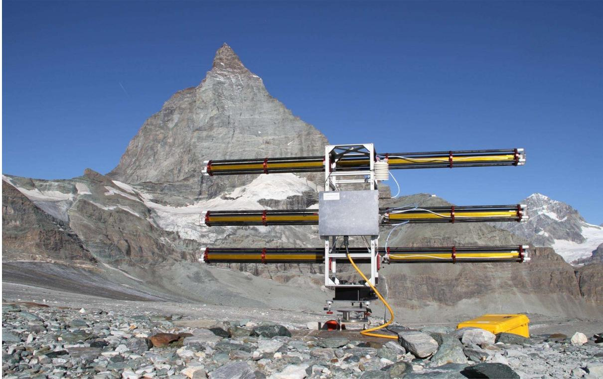
Figure 1: GPRI during observation of a slope instability at Matterhorn, Switzerland.
