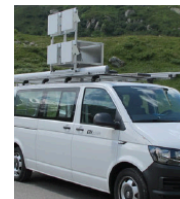
Car-borne setup of the L-band SAR system with one transmit and three receive antennas. Repeated SAR data acquisitions of the Stein Glacier were made while driving on a slightly curved section of mountain road.
