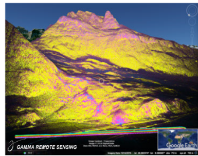
Google Earth view of UAV-borne L-band differential interferometric phase (left) and coherence (right) for nominally zero spatial baseline and a temporal baseline of 3 minutes. The flight tube of these two repeat-tracks are within 1m radius. With the exception of forested areas in the near range and areas with severe foreshortening a very high coherence is obtained and the interferometric phase is also stable.
