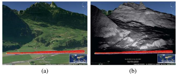
Fig. 3. a) Google Earth view of the UAV test site in Wolfenschiessen (CH). b) Geocoded intensity image overlaid to Google Earth view as obtained from a UAV-borne L-band SAR acquisition with a 2ms chirp duration focused with TDBP to a DEM-based reconstruction grid in map coordinates.
