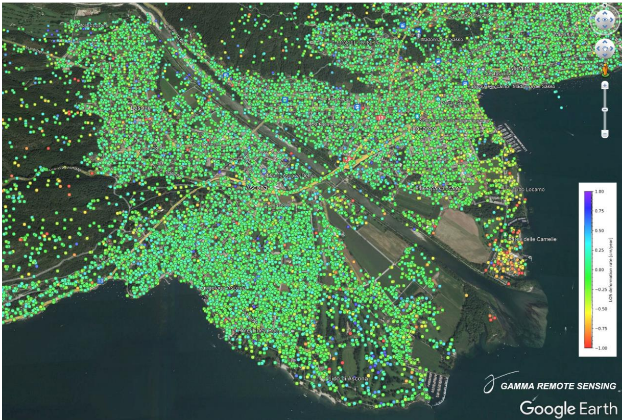
Figure 3 PALSAR-2 Persistent Scatterer Interferometry (PSI) over Locarno, Switzerland visualized in Google Earth.
